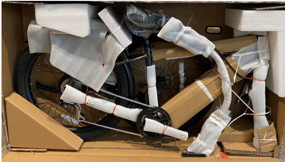
Figure 1: Bike frame, bike box, saddle, additional box of parts (Figure 2), front wheel, axle skewer, stem and handlebars, all zip tied together and padded.
